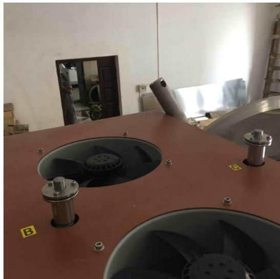
1-3. Regard the 3 assistant thermocouple, we equipped with plug. While it is not used, it can be blocked off. It also equipped with spare silicon ring. As shown below:
